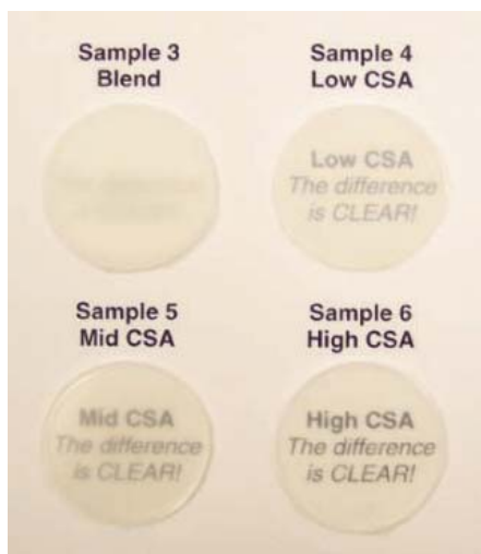
Fig. 3. Image of compression-molded samples (thickness = 0.35 \text{ mm} ), illustrating the effect of chain shuttling on clarity. Sample 3 is a physical blend of high- and low-density polymer and is opaque. Adding \text{Et}_2\text{Zn} during polymerization results in a block copolymer microstructure with intimately mixed interchain hard and soft segments, resulting in the increased transparency of samples 4 to 6.
